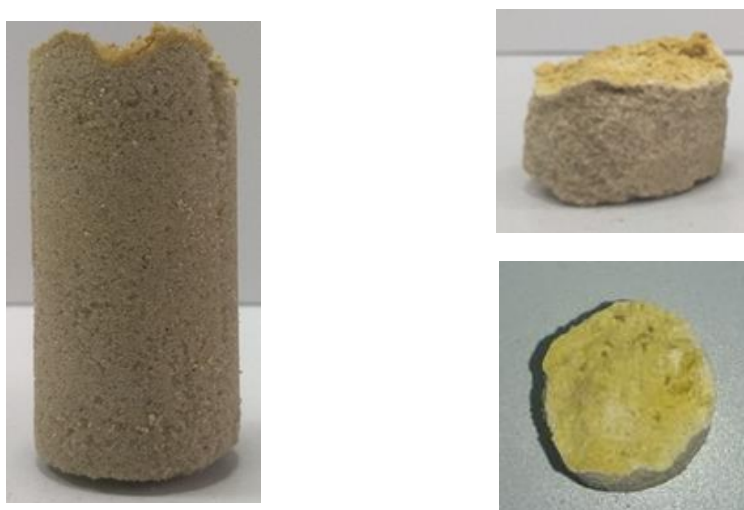
Figure 5. Sand after biocementation using soybean seed urease
