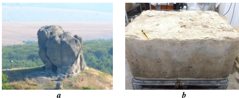
Figure 1. Object of natural biocementation: the rock in the village of Pidkamin, Ukraine (a) and the result of artificial biocementation using MICP of sand (b)
