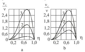
Figure 8. Dependence  $\frac{V_t}{V} = f(\eta)$  on the ratio (17) for water at  $t = 100 \ ^oC$ ,  $d = 0.02 \ m$ . a  $-u_2 = 10 \ m/s$ , 1 - Re = 1356; 2 - 4068; 3 - 6780. b -Re = 6780,  $1 - u_2 = 35 \ m/s$ ; 2 - 20; 3 - 0.
