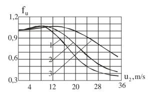
Figure 7. Dependence  $f_u = f(u_2)$  at Re = 6000 in the region of rarefaction: 1-  $\rho_2 = 0.6 \ kg/m^3$ ; 2 - 0,4; 3 - 0,2.
