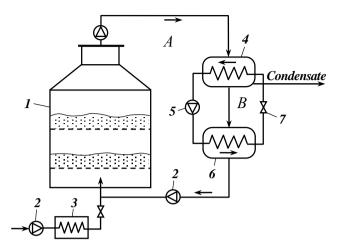
Figure 1. The scheme of the device for drying malt: A – contour of the drying agent; B – contour of thermal agent; 1 – dryer; 2 – fans; 3 – heater of drying agent; 4 – heat pump evaporator and condenser of steam of the drying agent; 5 – compressor; 6 – condenser of the heat pump; 7 – control valve
