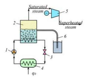
Figure 4. Heat pump circuit
