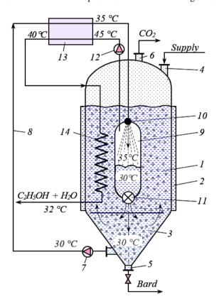
Figure 3. Scheme of the fermenter with a recuperative system of alcohol extraction
