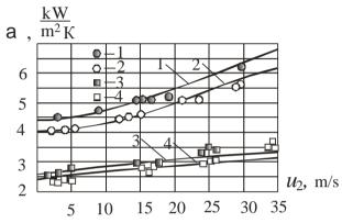
Figure 9. Dependence  $\alpha = f(u_2)$  for water and sugar solutions for the pipe, d = 20 mm.
