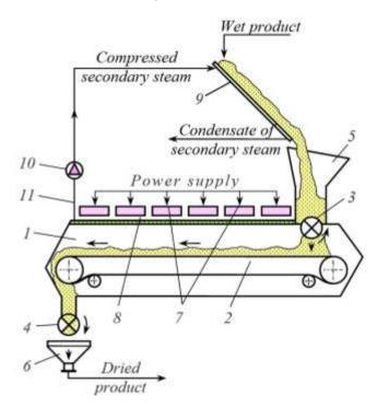
Figure 5. Scheme of a vacuum dryer of continuous action
