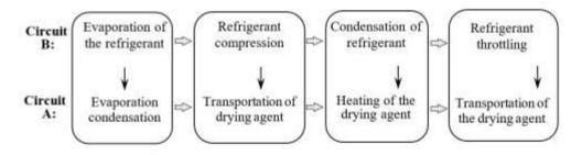
Figure 2. Synchronization of processes in the circuits A and B from Figure 1
