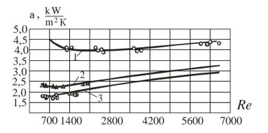
Figure 4. Dependence  $\alpha = f(\text{Re})$  for water and sugar solutions in a pipe with a diameter of 20 mm, length L = 1,5 m, t = 100 °C. 1 – water; 2, 3 – sugar solutions. 2 – DM = 40%; 3 – 50%.
