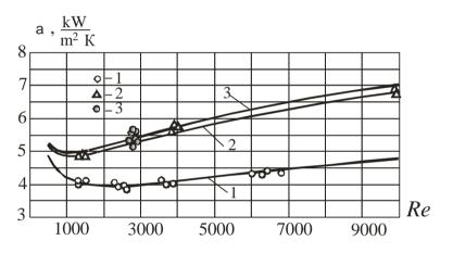
Figure 5. Dependence  $\alpha = f(\text{Re})$  for pipes of different diameters. 1 - data of the authors, d = 20 mm; 2 - d = 30 mm; 3 - data [12], d = 32 mm, water t = 100 °C.
