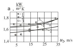
Figure 10. Dependence  $\alpha = f(u_2)$  for sugar solution with a concentration of 40% in a pipe
