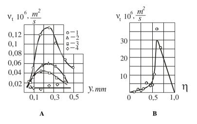
Figure 1. The dependence of turbulent viscosity on the film thickness of water (t = 20 °C). A – flow along an inclined angle of 9° (D.C. Jepsen); 1 – *Re* = 1834; 2 – 1462; 3 – 1099; 4 – 732, (method of CO<sub>2</sub> absorption);
